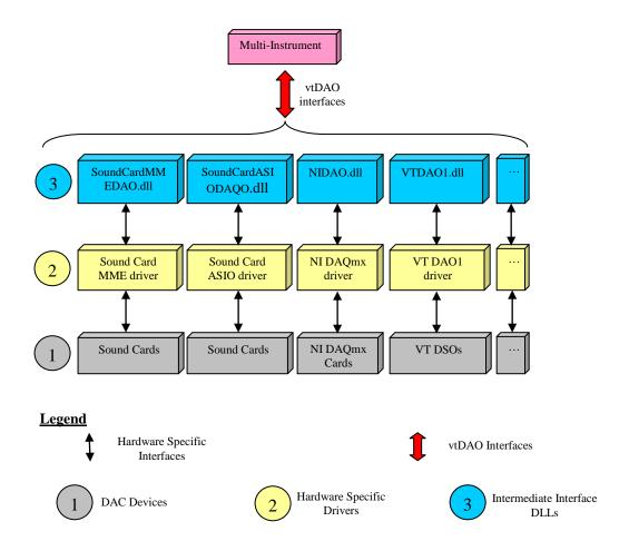
You can write your own back-end program to interface to the ADC and DAC devices that are supported by Multi-Instrument via vtDAQ and vtDAO interfaces. As all these devices conform to the same interface standard, you only need to write the interface codes in your program once and your program will support all these devices.
