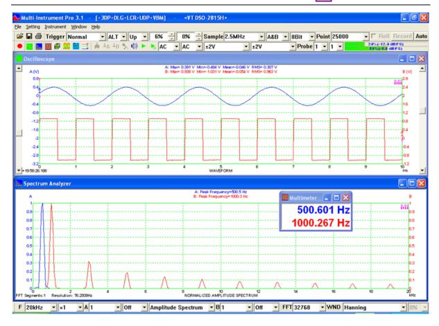
The following figure is a mixed signal display. Channels A & B are analog input channels while Channel EXT is used as a digital input channel.
