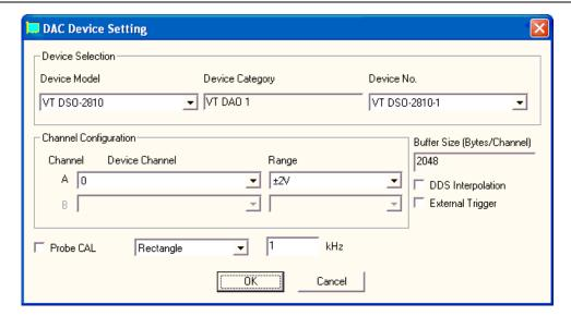
You can choose to output either Rectangle or MLS signal. When MLS is selected, the frequency value here refers to the clock frequency of the MLS generator rather than the output signal frequency. By default, the Probe CAL signal output is enabled. You can disable the signal output by un-ticking the "Probe CAL" checkbox. This will help to improve the Signal-to-Noise ratio in the oscilloscope, especially when the measuring range is lower than 100 mV.
