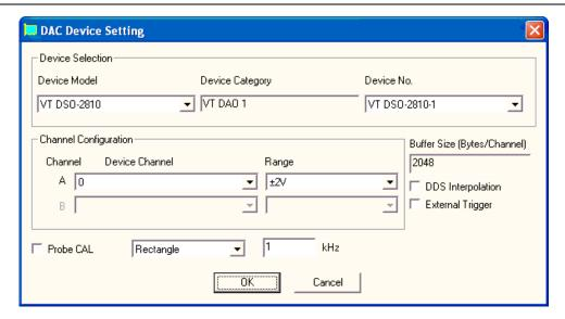
You can choose to output either Rectangle or MLS signal. When MLS is selected, the frequency value here refers to the clock frequency of the MLS generator rather than the output signal frequency. By default, the Probe CAL signal output is enabled. You can disable the signal output by un-ticking the "Probe CAL" checkbox. This will help to improve the Signal-to-Noise ratio in the oscilloscope, especially when the measuring range is lower than 100 mV.
