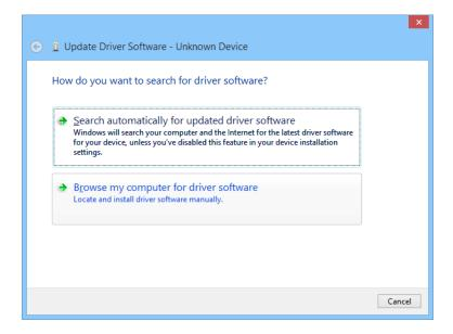
4) Choose "Search for driver software in this location" and "Browse...", and then locate the driver. The driver can be found at Multi-Instrument's installation directory\Drivers\VTUSB3\32bit or 64bit. Choose 32-bit or 64-driver according to your Windows version. After that, press "Next".
