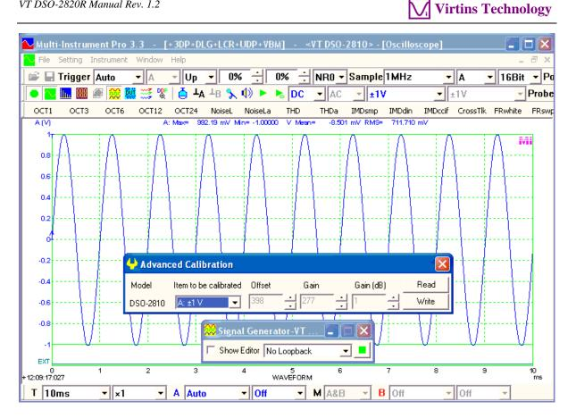
You can calibrate the offset and gain settings for each voltage measuring range and for each channel. The following are the steps to calibrate Channel A at  $\pm 1V$ .
