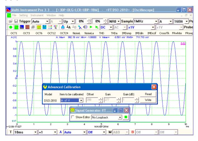
You can calibrate the offset and gain settings for each voltage measuring range and for each channel. The following are the steps to calibrate Channel A at  $\pm 1$ V.
