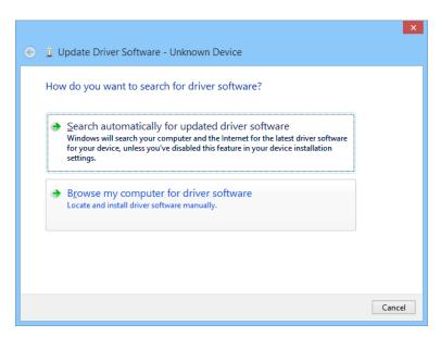
4) Choose "Search for driver software in this location" and "Browse...", and then locate the driver. The driver can be found at Multi-Instrument's installation directory\Drivers\VTUSB3\32bit or 64bit. Choose 32-bit or 64-driver according to your Windows version. After that, press "Next".
