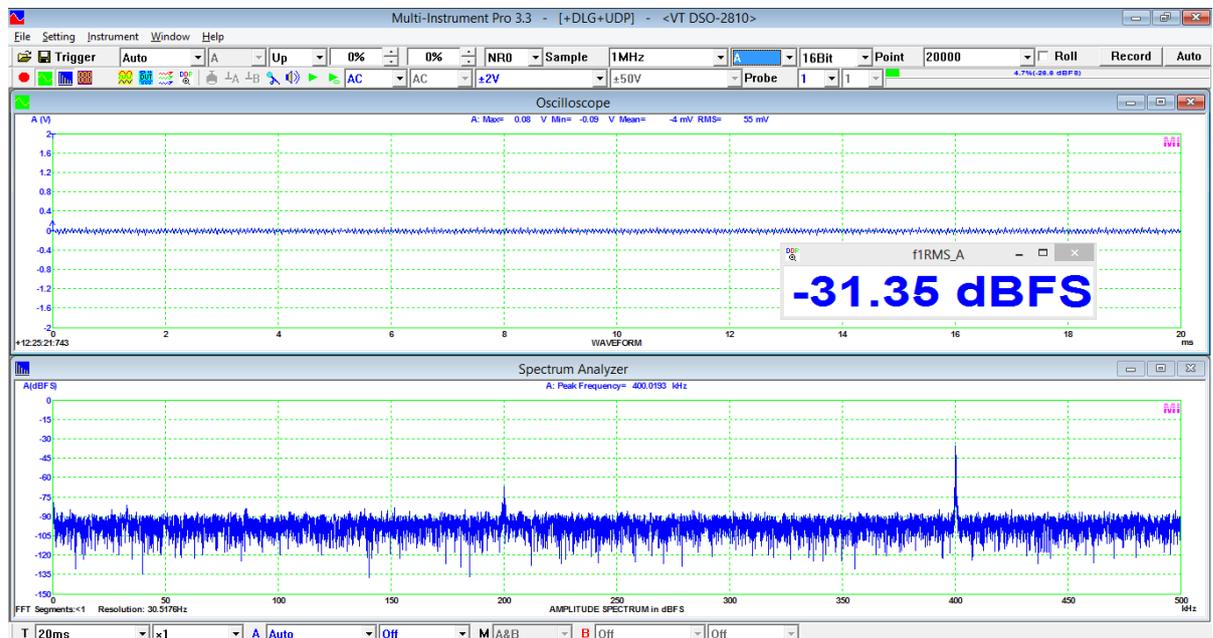
$f_s = 1 \text{ MHz}$ , 4.4 MHz appears as 400 kHz due to aliasing, 16-Bit Mode, magnitude = -31.35 dBFS, decreased 22.83 dBFS as compared with that of 8-Bit Mode thanks to the adaptive anti-aliasing filter
