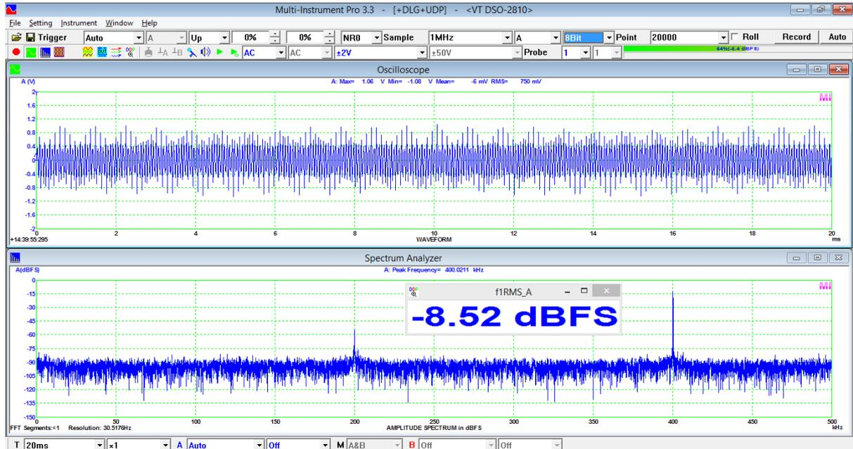
$f_s = 1 \text{ MHz}$ , 4.4 MHz appears as 400 kHz due to aliasing, 8-Bit Mode, magnitude = -8.52 dBFS
