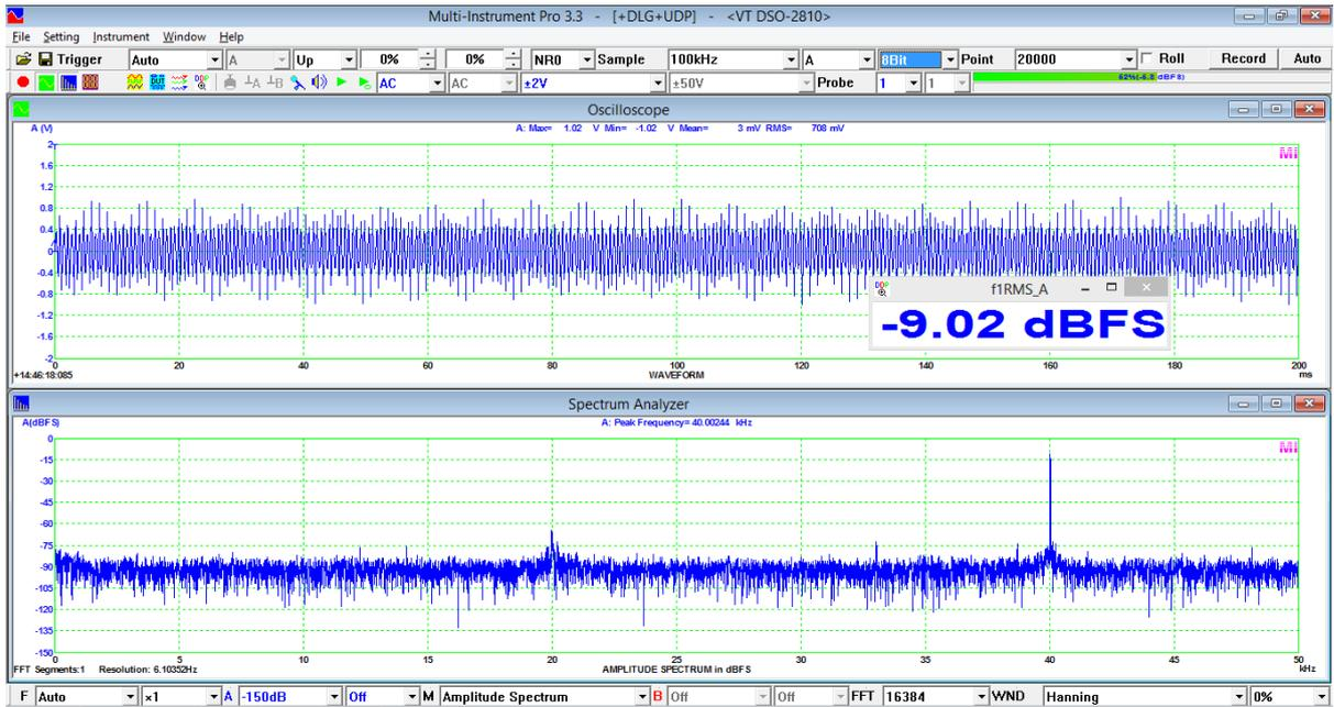
$f_s = 100$  kHz, 440 kHz appears as 40 kHz due to aliasing, 8-Bit Mode, magnitude = -9.02 dBFS
