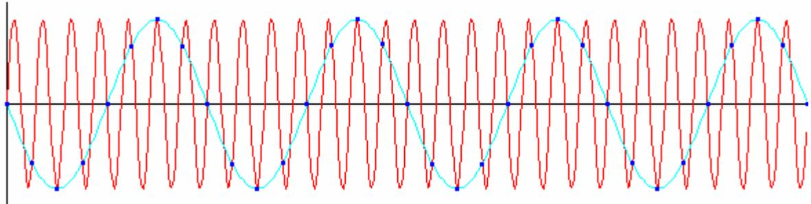
The only solution to the aliasing problem is to ensure that the sampling rate is higher than twice of the highest frequency present in the signal. If that is not possible, then use an anti-aliasing filter to screen out those frequencies higher than  $1/2$  of the sampling frequency before sampling, assuming the removed frequencies are not of importance.
