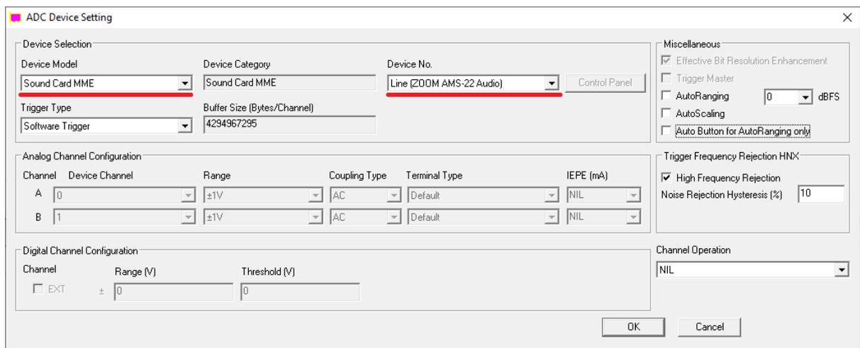
Note that the displayed name of the sound card may vary a bit under different Windows versions or with different USB ports.
