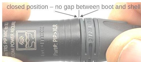
Use the reverse procedure to remove adapter.
