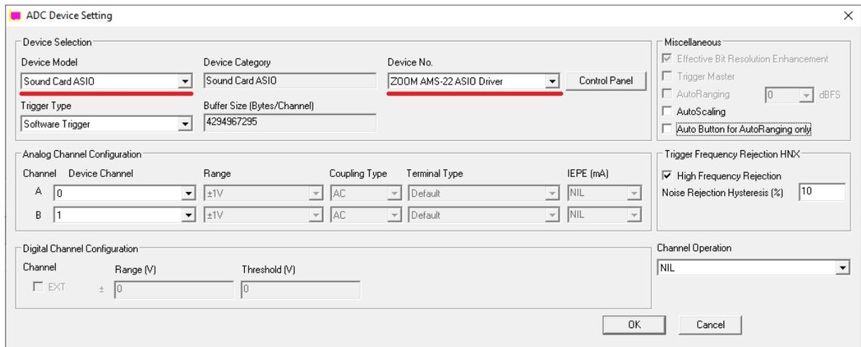
Now, if you start the oscilloscope by pressing the red button at the upper left corner of the screen, and then talk LOUDLY before the hydrophone, you should be able to see your “voices” in the Oscilloscope and Spectrum Analyzer.
