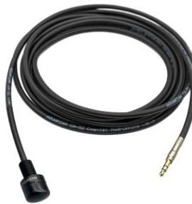
The 3.5mm TRS plug can be connected directly to a standard 3.5mm mic jack that supplies plug-in power (PIP) (2.4V, min. 400 $\mu$ A). It is wired dual mono: tip and ring (output), sleeve (ground). The outside diameter is 5.5mm.
