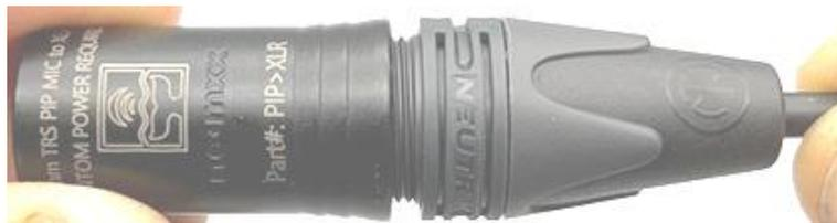
Tighten the chuck by turning the boot clockwise until snug. Hand tighten only. Note that there should be no gap between boot and XLR connector shell when tight. Test by gently pulling on the hydrophone cable.
