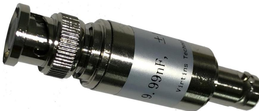
VT CAP is a precision capacitor epoxy-sealed inside a metal case with BNC connectors at both ends. It can be used in series with a voltage signal generator in order to simulate charge output during calibration or checking of a charge amplifier. The capacitor has a low dissipation factor, low dielectric absorption coefficient and very constant capacitance against temperature and humidity variation.
