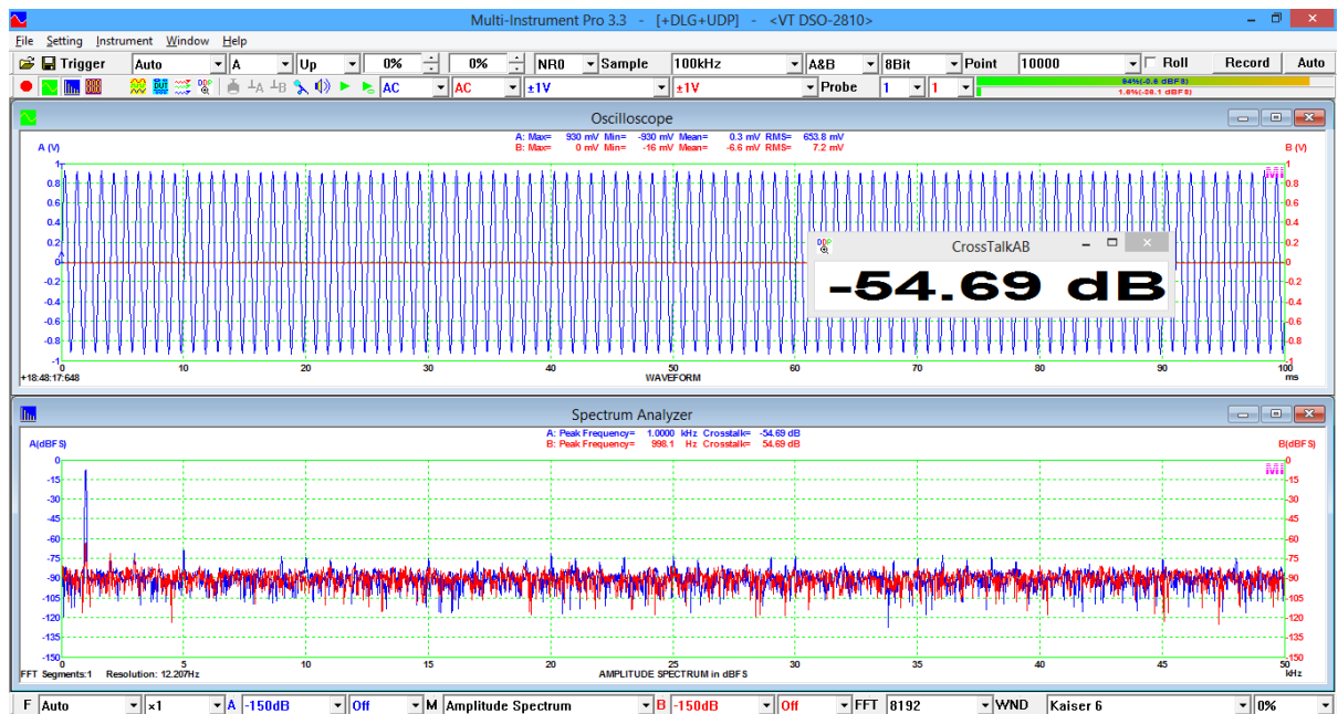
Crosstalk Measurement of a VT DSO-2810, Enhanced 8-Bit Mode f_s=100\text{kHz} , f=1\text{kHz} , full-scale input
