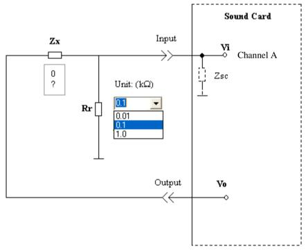
where: Rr is the reference resistor. Zx is the impedance to be measured. Zsc is the sound card input impedance. Vo is the output RMS voltage. Vi is the input RMS voltage.
