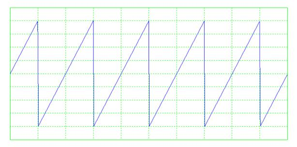
A saw tooth waveform will be generated. Note that the above figure also illustrates the initial phase of the generated signal.
