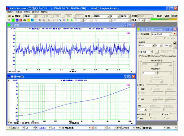
The following figure shows a periodic noise signal generated using SpeechMale.frf. It can be used as the male Speech Transmission Index test signal according to IEC 60268-16.
