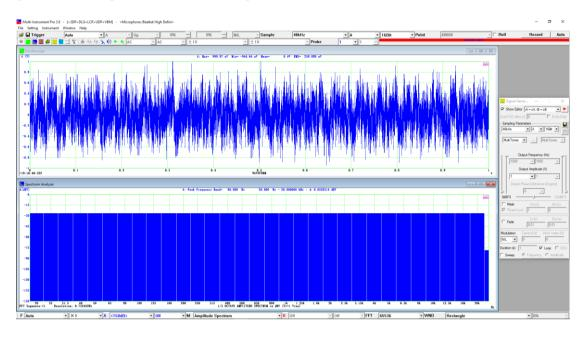
Both of the above two figures have a perfectly flat spectrum in the range of 20 Hz  $\sim$  20 kHz under 1/3 octave analysis with a rectangle window function. However, the former shows some patterns (unwanted sometimes) in time domain while the latter does not.
