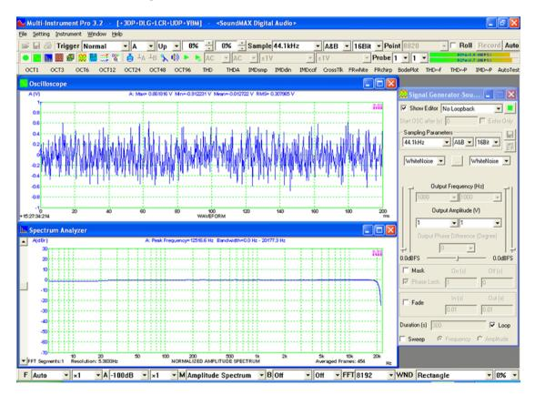
The following figure illustrates the bandwidth of an EMU Tracker Pre USB sound card measured using an external loopback cable. The measured bandwidth is about 7.3Hz ~ 90443Hz when the sampling rate is 192 kHz. White noise was used as the stimulus and 200 frames were averaged.
