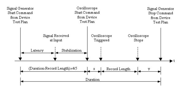
x+y in the above figure accounts for 1/5 of [Duration – Record Length]. The trigger condition should be set properly such that y is greater than zero. If you set the Trigger Edge to "DF", Trigger Level to "0" and Trigger Delay to "0", then x will be 0. Difference DUT and ADC/DAC device have different latency and require different time to get stable, thus designing a correct timing scheme is critical for the SIO instruction.
