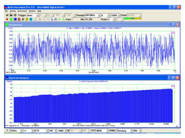
By default, the generated white noises in different channels are not correlated. To generate identical white noises in both channels, tick "Same Across Channels" checkbox in the following figure.
