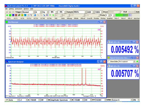
The following figure illustrates the CCIF3 IMD of a laptop built-in sound card measured using an external loopback cable.
