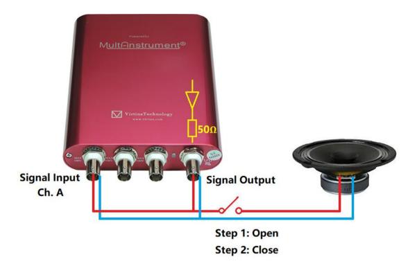
Under the impedance measurement mode, Channel A Display Range and Channel B Display Range will be updated to display impedance in  $\Omega$ . The display range of the "Auto" option is about 5×Rr. The following DDPs are generated by this mode:
