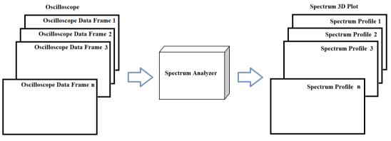
Inter-frame Mode of Spectrum 3D Plot - STFT
