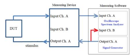
Single-Channel Method (iB=0A) for Transfer Function / Impulse Response Measurement
