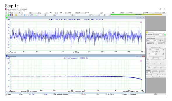
The above figure actually shows the overall frequency response of the setup. It mainly reflects the fact that VT DSO-2A20E's anti-aliasing filter has a cutoff frequency at  $0.443 \times [\text{Sampling Frequency}] = 0.443 \times 50 \text{ kHz} = 22.15 \text{ kHz}$  under its 16-bit mode. Note that there is no need to compensate the frequency response in this test.
