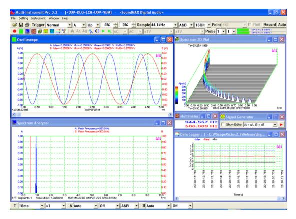
VIRTINS<sup>®</sup> Multi-Instrument is a powerful multi-function virtual instrument software. It is a professional tool for time, frequency, time-frequency and modulation domain analyses. It supports a variety of hardware ranging from sound cards which are available in almost all computers to proprietary ADC and DAC hardware such as NI DAQmx cards, VT DSO, VT RTA, VT IEPE, VT CAMP, RTX6001 and so on. It consists of the following instruments and functions.
