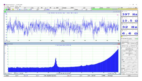
The measured resonant frequency is 397 Hz at the impedance peak 10.5  $\Omega$ . The lowest impedance is 6.6  $\Omega$  at the lower frequency end.
