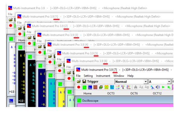
If multiple instances point to the same hardware device (either the same or different channels), the device driver must support multi-client applications, otherwise, clash will occur. Sound card MME drivers and some sound card ASIO drivers support multi-client applications, but VT DSO drivers do not.
