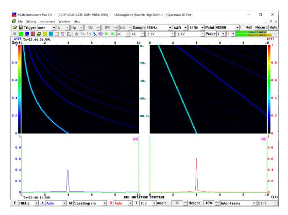
The toggle button in the Instrument Toolbar is used to open or close the Spectrum 3D Plot. The button is enabled only when the Spectrum Analyzer is under Amplitude Spectrum mode, because the spectral profiles are fed from the Spectrum Analyzer under that mode. All intra-frame processing options set in the Spectrum Analyzer are applicable to the Spectrum 3D Plot too.
