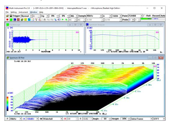
The data in the above figure can be exported to EXCEL for further analysis. The exported data can be either time-sliced or frequency-sliced. The following figure shows the sound pressure level decay in the 1kHz 1/1 octave band using the exported frequency-sliced data.
