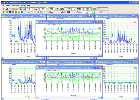
This is a dual channel parameter data logger. It provides long time data logging function for 246 derived data points and 16 user defined data points, including RMS value, Peak Frequency, Sound Pressure Level, RPM, THD, etc. Up to eight data logger windows can be opened and each window can trace up to 8 variables. The logged data can be reloaded for review.
