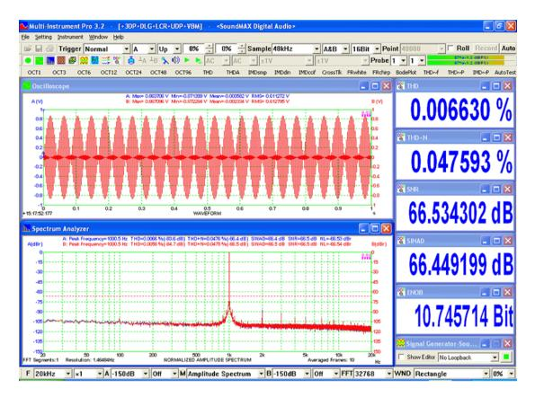
The following figures shows the THD related parameters of the same laptop built-in sound card measured via a loopback at the sound card's mixer level. As you can see that all the parameters are substantially better than the above case, due to the fact that the current measurement excluded the adverse contribution from the sound card's power amplifier (output) and mic amplifier (input) as well as the possible external noises induced via the external loopback cable.
