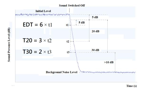
T20 is the RT60 derived from the decay curve between 5dB and 25dB below the initial level. The initial level must be at least 35dB higher than the background noise level.
