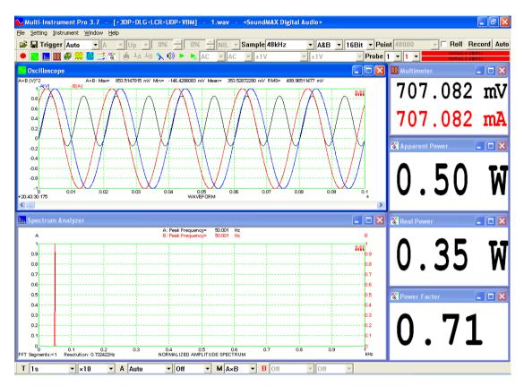
2.5.5.5 A/B (XY Mode, Lissajous Pattern) Lissajous Pattern display for Channel A and Channel B.
