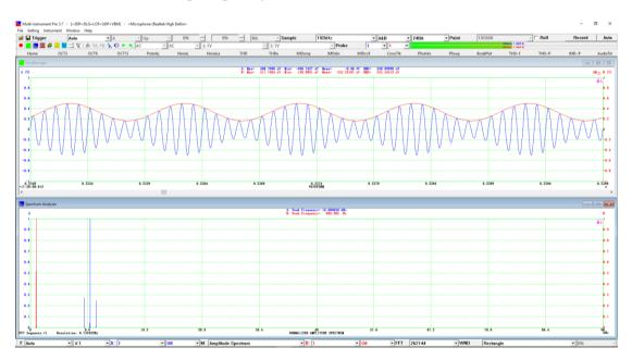
"Remove DC" or a high pass filter (described later) can be used to remove the DC component in the demodulated signal in the above figure. When AM demodulation is applied to a channel, the symbol "AM" will be displayed beside the corresponding axis label in the Oscilloscope view.
