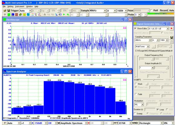
The gender-specific spectra of STI test signals are defined in IEC 60268-16 as follows.
