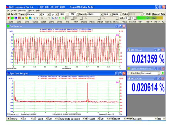
The following figure illustrates the DIN IMD of a laptop built-in sound card measured using an external loopback cable.
