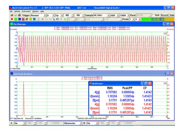
Both SI and English unit systems are supported. The software will automatically choose the unit system according to the sensor sensitivity units entered via [Setting]>[Calibration]>"Sensor">"Unit". Manual switching between the two unit systems is only allowed when acceleration sensors are used.
