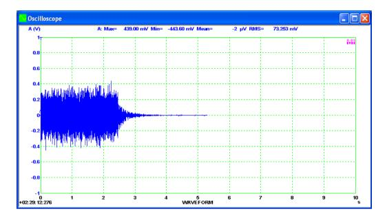
During reverberation analysis, the directly recorded instantaneous sound pressure variation will be band-pass filtered for each frequency band of interest and converted to sound pressure level (dBSPL) with the integration time determined by the software automatically (see figure below). EDT, T20 and T30 will then be calculated automatically according to ISO3382. Note that the latter two are obtained through linear regression.
