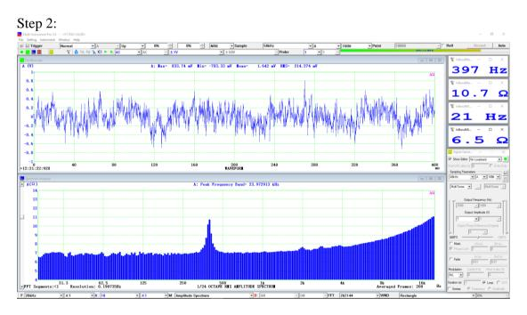
The measured resonant frequency is 397 Hz at the impedance peak 10.7  $\Omega$ . The lowest impedance is 6.5  $\Omega$  at the lower frequency end.
