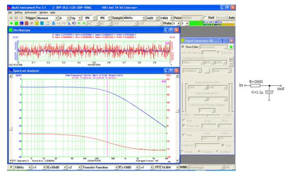
The following DDPs are generated by the transfer function display mode:
