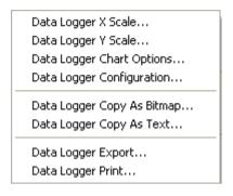
Data Logger does not have its own menu and view parameter toolbar. Its functions are accessed via its context menu. The context menu pops up when you right click anywhere within the data logger window.
