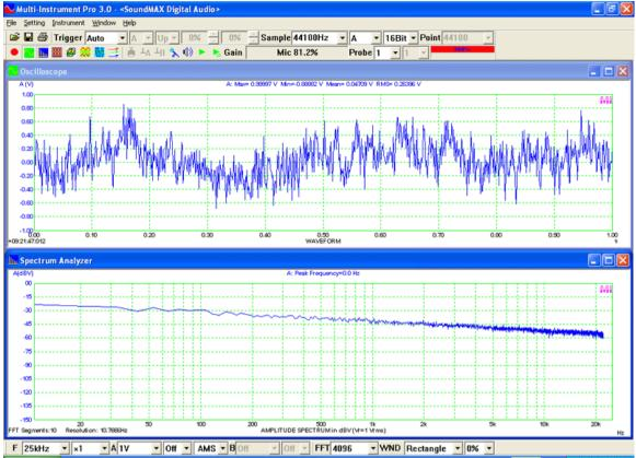
The following figure is the 1/12 octave amplitude spectrum (in dBV) of the same pink noise. It shows that the spectrum is rather flat in octave scale.
