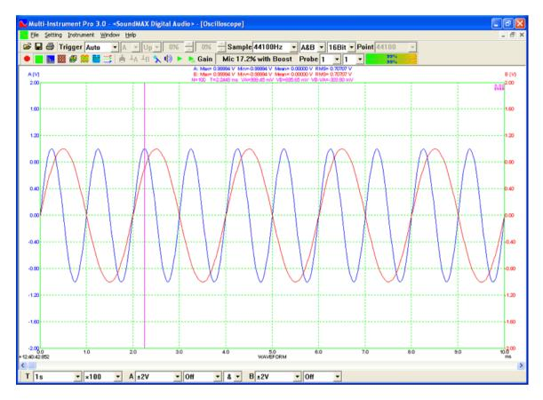
The cursor reader is shown when you left click and hold anywhere within the plot region of a view. It will stick to the actual measurement point nearest to the cursor in the horizontal direction and show its X and Y readings for both channels in the top region of the view. The cursor reader moves with the cursor and remains active until the left mouse button is released.
