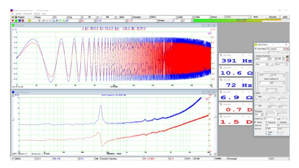
The measured resonant frequency is 391 Hz with an impedance peak of 10.6  $\Omega$ . The lowest impedance is 6.9  $\Omega$  at the lower frequency end. The phases at the resonant frequency and lower frequency end are 0.7 degree and 1.5 degree respectively, which are very close to zero.
