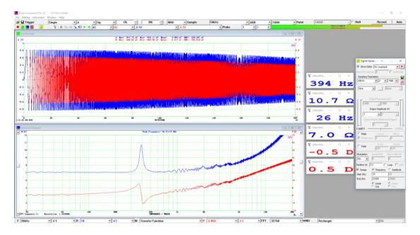
The measured resonant frequency is 394 Hz with an impedance peak of 10.7  $\Omega$ . The lowest impedance is 7.0  $\Omega$  at the lower frequency end. The phases at the resonant frequency and lower frequency end are -0.5 degree and 0.5 degree respectively, which are very close to zero.
