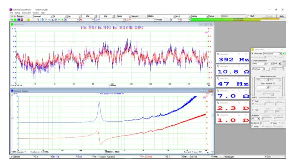
The measured resonant frequency is 392 Hz with an impedance peak of 10.8  $\Omega$ . The lowest impedance is 7.0  $\Omega$  at the lower frequency end. The phases at the resonant frequency and lower frequency end are 2.3 degree and 1.0 degree respectively, which are very close to zero.
