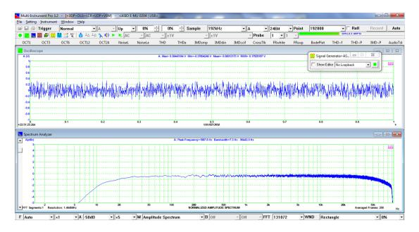
Bandwidth can be accessed through these DDPs: BandWidthLowLimit\_A(Hz) and BandWidthHighLimit\_A(Hz) for Channel A, and BandWidthLowLimit\_B(Hz) and BandWidthHighLimit\_B(Hz) for Channel B. They can also be used to derive Quality Factor and Damping Ratio.
