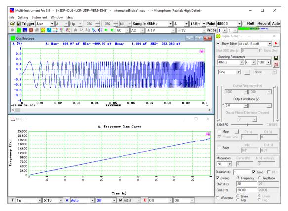
This DDC is derived from one frame of Oscilloscope data.
