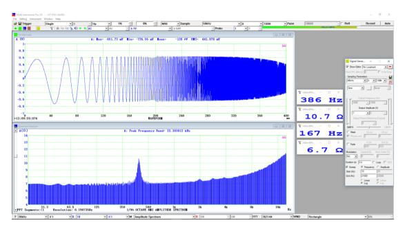
The measured resonant frequency is 386 Hz at the impedance peak 10.7  $\Omega$ . The lowest impedance is 6.7  $\Omega$  at the lower frequency end.
