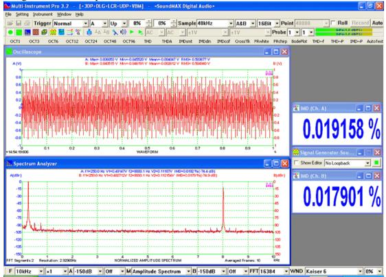
The following figure illustrates the CCIF2 IMD of a laptop built-in sound card measured using an external loopback cable.
