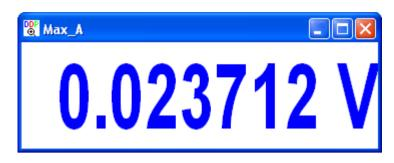
DDP viewer is used to display the value of a DDP (Derived Data Point) in a dedicated window with a bigger font size. It is also possible to specify the DDP's high-high, high, low, low-low limits for alarming and the number of decimal places for display. Different alarm sounds can be configured for different types of alarms. Alarm acknowledgement is supported. Up to 32 DDP viewers can be opened. These DDP viewers can also be used to define and display UDDPs (User Defined Data Points)
