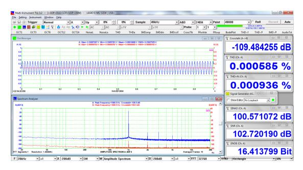
Crosstalk can be accessed through these DDPs: CrossTalkAB(dB) for crosstalk from Channel A to Channel B and CrossTalkBA(dB) for crosstalk from Channel B to Channel A. Some recommended panel settings for crosstalk measurement are provided in the Panel Setting File (PSF) directory of the software.
