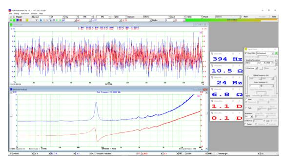
The measured resonant frequency is 394 Hz at the impedance peak 10.5  $\Omega$ . The lowest impedance is 6.8  $\Omega$  at the lower frequency end. The phases at the resonant frequency and lower frequency end are 1.1 degree and 0.1 degree respectively, which are very close to zero.
