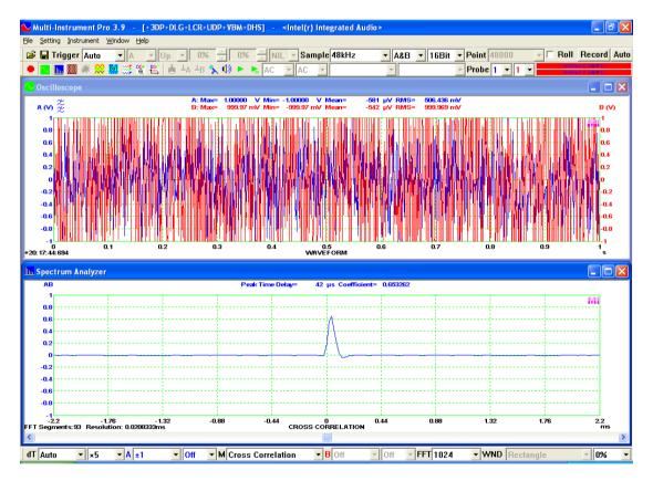
The impulse response (or circular cross correlation) data in the above figure can be exported to a TXT file by right clicking anywhere within the Spectrum Analyzer and select [Spectrum Analyzer Export]. It can then be imported via [File]>[Import] into the Oscilloscope in order to show its magnitude frequency response in the Spectrum Analyzer (see figure below). It can be seen from the figure that the -3dB cutoff frequency of the low pass filter is correctly measured to be 5513Hz.
