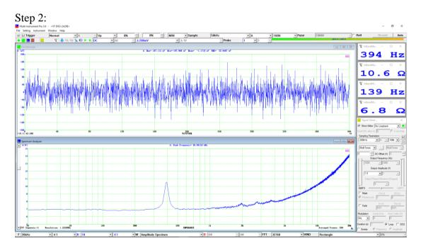
The measured resonant frequency is 394 Hz at the impedance peak 10.6  $\Omega$ . The lowest impedance is 6.8  $\Omega$  at the lower frequency end.
