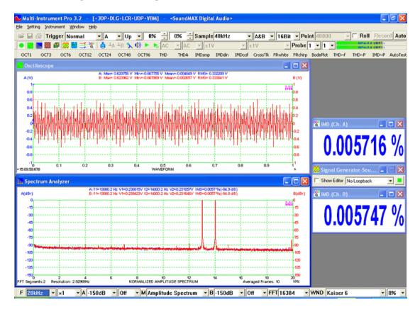
Some professional sound cards in the market have excellent performances in audio parameter measurements. The following figure illustrates the SMPTE IMD of an EMU Tracker Pre USB sound card measured using an external loopback cable.
