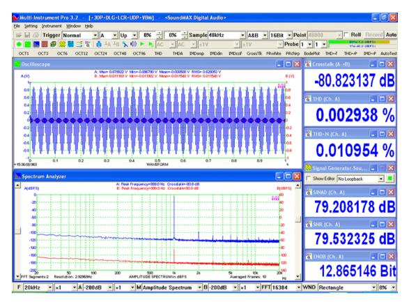
The following figure illustrates the crosstalk at 1 kHz from Channel A to Channel B of an EMU Tracker Pre USB sound card measured using an external loopback cable. The crosstalk is about -109dB.
