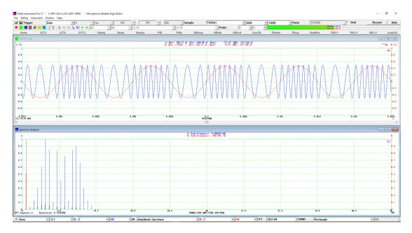
Multi-Instrument features unique FM demodulation algorithm which is able to demodulate the FM signal accurately even when the sampling rate is not very high compared with the FM signal spectrum.
