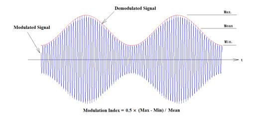
To measure the amplitude modulation index (or amplitude modulation depth), the modulated signal needs to be demodulated first. Then the modulation index can be obtained as follows:
