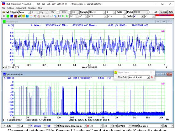
Generated without "No Spectral Leakage" and Analyzed with Kaiser 6 window
