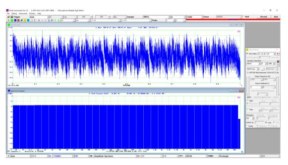
The following figure shows the 1/3 octave amplitude spectrum (in dBV) of a multitone signal aligned to 1/3 octave bands in the range of 20 Hz ~ 20 kHz, generated using the automatic configuration method instead.
