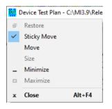
"Sticky Move" option can be accessed by clicking the icon at the upper left corner of the Device Test Plan panel. It is ticked by default. With this option selected, all X-Y Plots will move together if you drag the title bar of the Device Test Plan panel.
