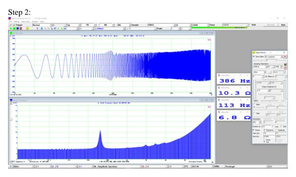
The measured resonant frequency is 386 Hz at the impedance peak 10.3  $\Omega$ . The lowest impedance is 6.8  $\Omega$  at the lower frequency end.
