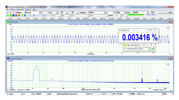
In addition to the IMD values, the two test tone frequencies and their RMS values measured will also be displayed. The test tone frequencies here are measured with a sub-FFT-bin-size accuracy. IMD can be accessed through the DDPs:  $IMD_A(\%)$  and  $IMD_A(dB)$  for Channel A and  $IMD_B(\%)$  and  $IMD_B(dB)$  for Channel B.
