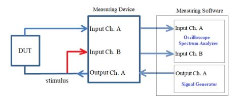
Dual-Channel Method (no software loopback) for Transfer Function / Impulse Response Measurement
