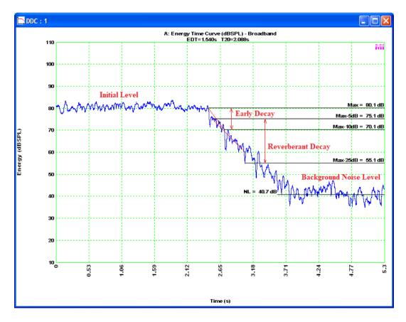
The decay curve measured with this method may vary from one measurement to another with no change in the characteristics of the enclosure and transmitting /
