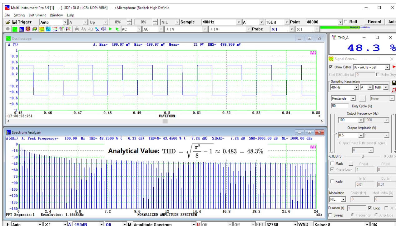
Fig. 48 Measured and Analytical THD of A Square Wave
