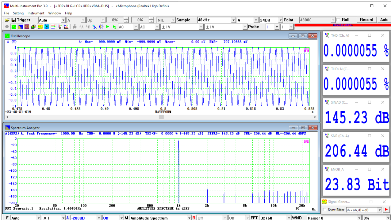
Fig. 3 Non Full-cycle Sampling with a Kaiser 8 window suppressing greatly spectral leakage
