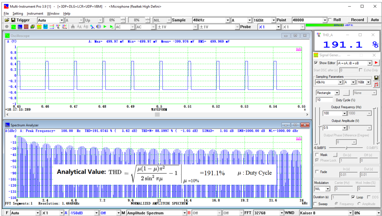
Fig. 51 Measured and Analytical THD of A Rectangle Wave (Duty Cycle =10%)
