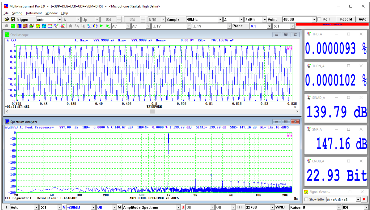
Fig. 21 [Sampling Rate] = 48 kHz, [Signal] = 997 Hz + 2991 Hz with Amplitude Ratio 1: 0.0000001, [FFT Size] = 32768, [Window] = Kaiser 8 (Simulation)
