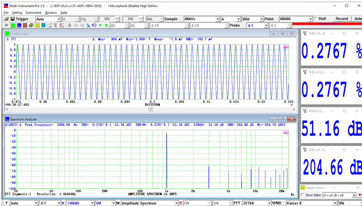
Fig. 5 An Integer Ratio of Sampling Rate to Signal Frequency ( 48000 / 1000 = 48 ) Concentrates Quantization Noise at Signal Harmonics (8 Bits)
