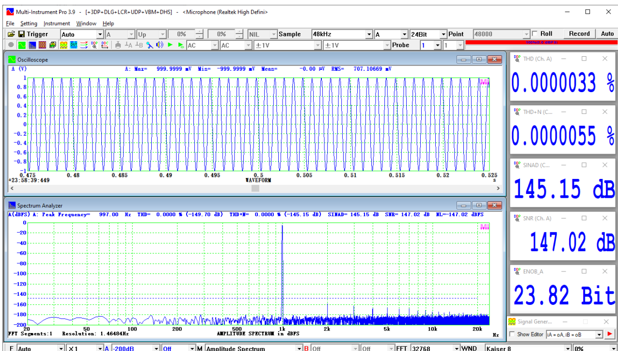
Fig. 4 A Non-Integer and Non-irreducible Ratio of Sampling Rate to Signal Frequency ( 48000 / 997 = 48.144433 ) Randomizes Quantization Noise (24 Bits)
